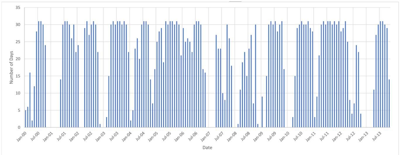
Figure 15: days during the months of 2000–13 where Sandford Hydro could be expected to be below full flow capacity
