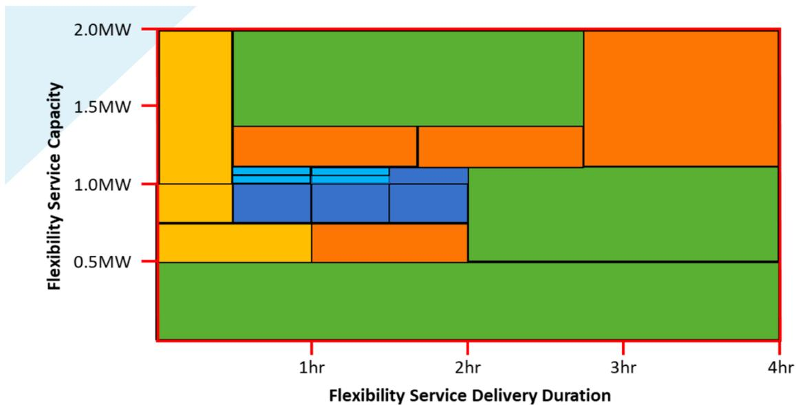
Figure 9: how a portfolio of different assets can work together to deliver a flexibility service (the different colours each represent a different DER)
