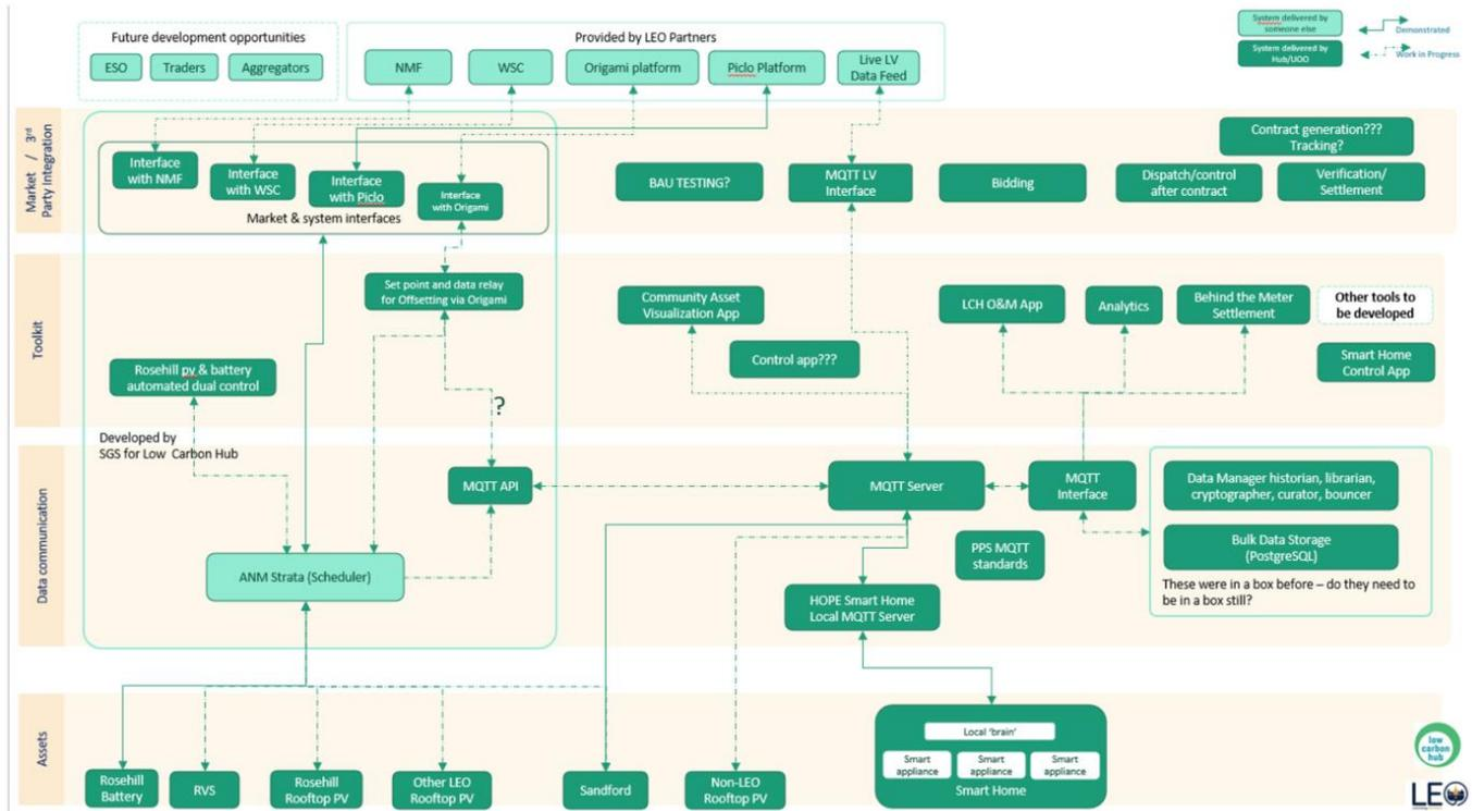
Figure 21: PPS 2.0 technical configuration: ANM Strata (left-hand side) and Internet of Things (right-hand side)
