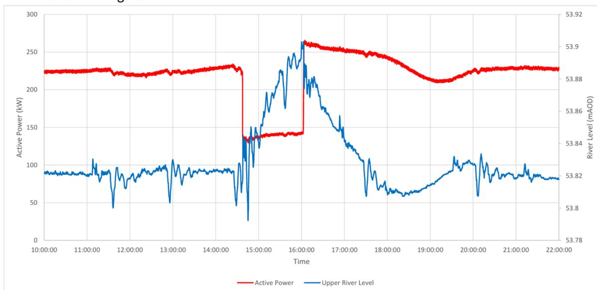
Figure 17: an example of the power output and river flow response at Sandford Hydro during the delivery of a flexibility service requiring the upturn of generation
