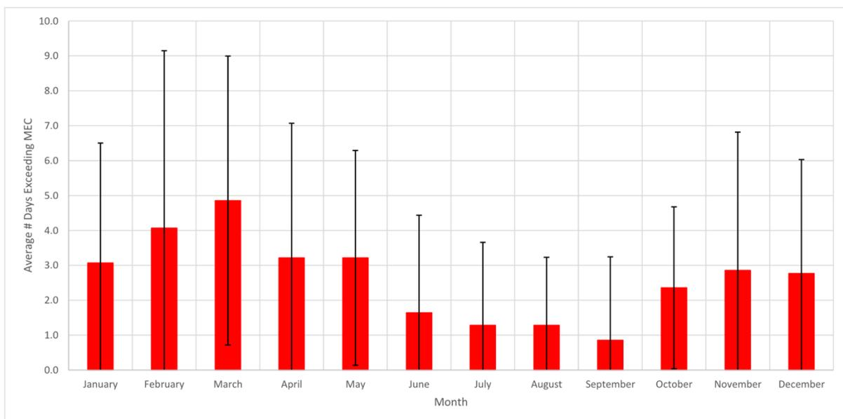
Figure 18: average number of days per month where the average Sandford Hydro power output would exceed the MEC based on historic data from 2000–13
