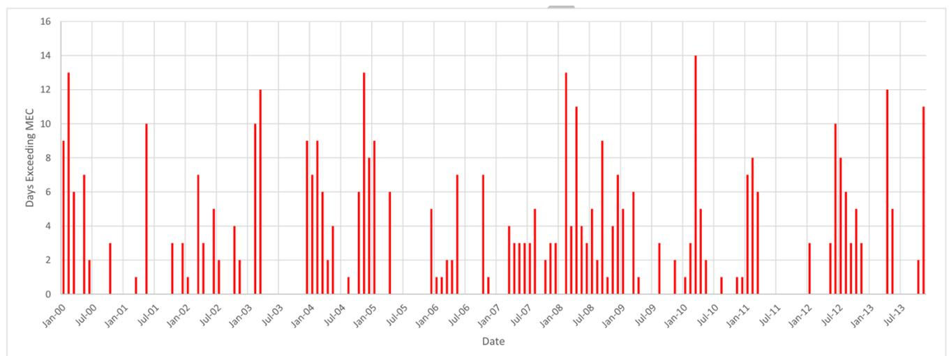
Figure 19: days during the months of 2000–13 where the average power output of Sandford Hydro would be expected to exceed the MEC
