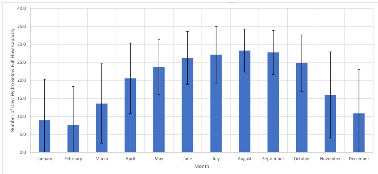
Figure 16: average number of days where Sandford would be below full capacity based on river flow data from 2000–12
