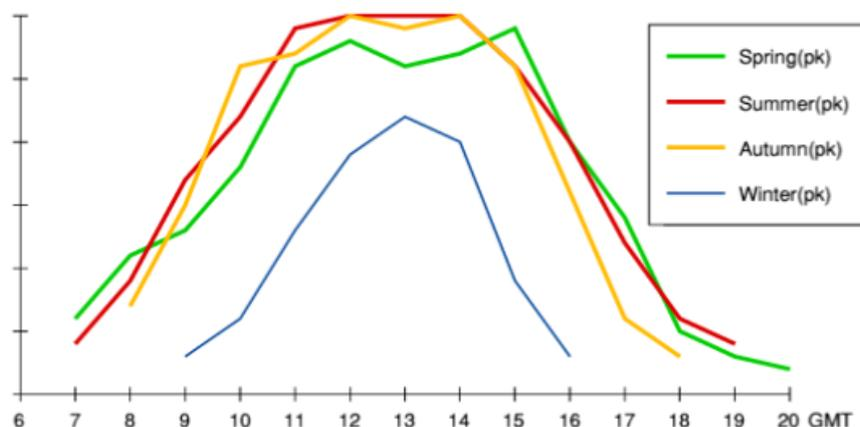
Figure 20: solar generation curve example
