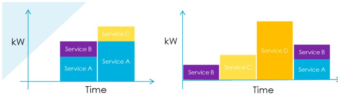
Figure 8: the difference between coincident delivery on the left and adjacent delivery on the right
